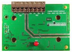
Figure 1: 4090-5206 Line Isolator Module
